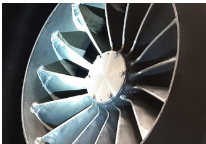
Paraformaldehyde deposits on fan impeller
